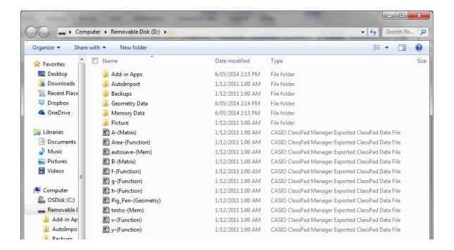
The exported files will now appear in .xcp format in the folder view on your connected computer, as illustrated above. They may now be transferred to your computer, in the same method as before by connecting the USB cable and selecting the USB Flash option on your CLASSPAD.
