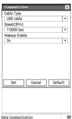
The Cable Type must be set to USB Cable to communicate with a computer, and 3-pin for communication between calculators.
