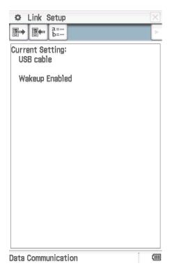
If the Current Setting is not USB cable and Wakeup enabled, select 'Open Setup' from the Setup Menu.
